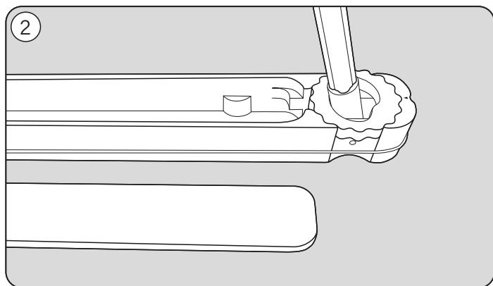
1. Move the elastic band to one side of the case. Remove the cover and adjustment wheel.
